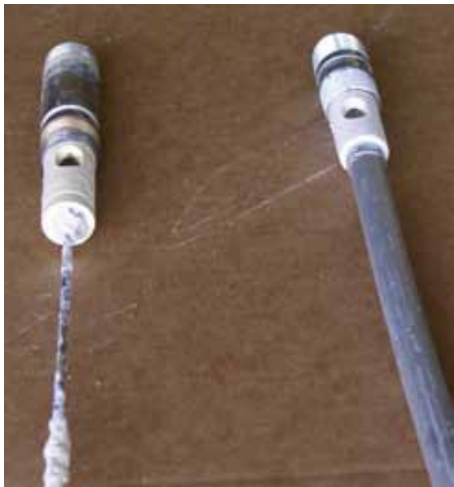
Old and new anode rods.
